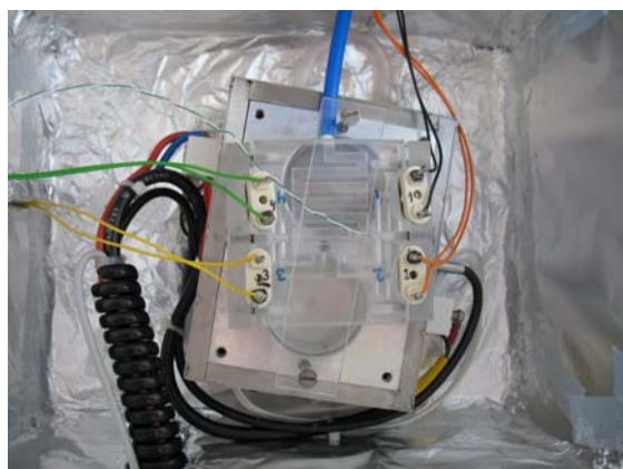
Figure 7: Flow system with temperature and flow control. Four QCMs can be characterized simultaneously.
